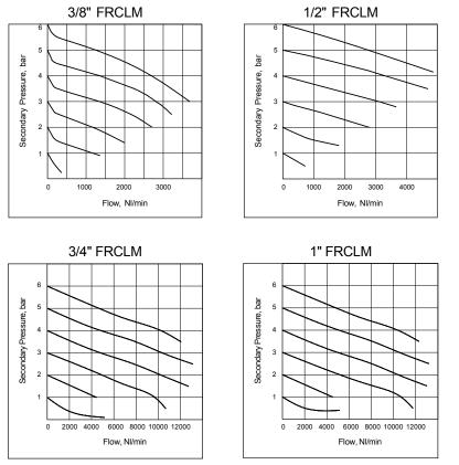
Flow graphs are for 40µm filterations only
