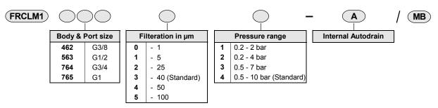
Ordering example : Filter Regulator Combination and Lubricator Modular - 3/8 size ( with G3/8 port ) with 5µm Filter and pressure range 0.5 - 7 bar with Internal Autodrain : Ordering No : FRCLM146213-A/MB.
